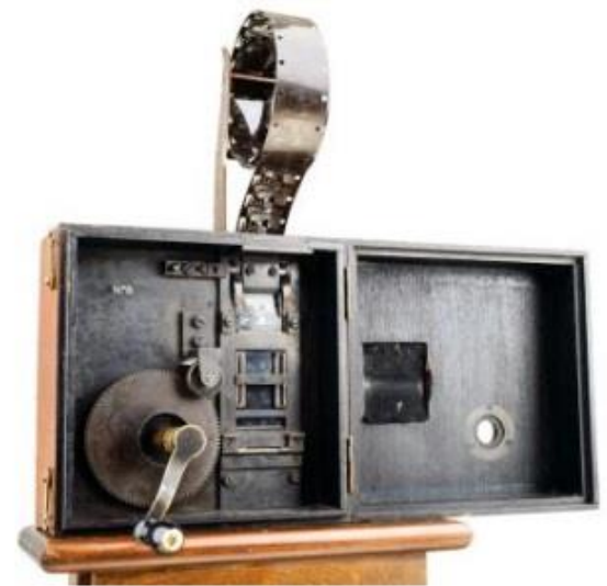
Cinématograph patented by the Lumière brothers in 1895
